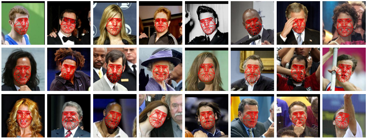
Fig. 7: Face alignment examples in the Labeled Faces the Wild dataset [40] taken using the BCLM-KDE fitting algorithm.
