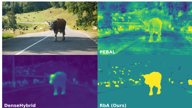
Figure 1: Preserving objectness and eliminating noise. While state-of-the-art methods PEBAL [65] and DenseHybrid [25] suffer from a lack of smoothness and objectness with high false positive rates, our method RbA clearly segments the unknown objects and reduces false positives by eliminating uncertainty at semantic boundaries and in ambiguous background regions.
