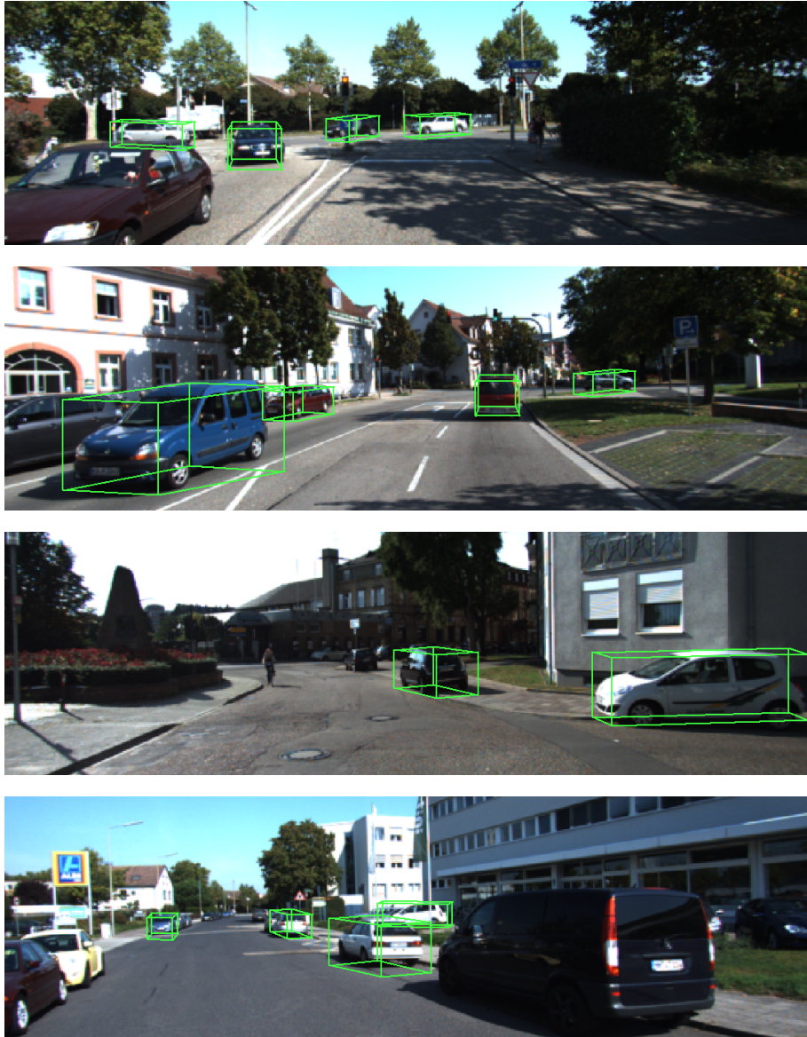
Figure 6.6: Example detections and visualization of estimated poses in the KITTI dataset. The pose is determined by the facing angle of a car along the vertical axis, representing an out-of-plane rotation. An illustration of the predicted pose is presented as a rotated 3D bounding box. Best viewed in color.
