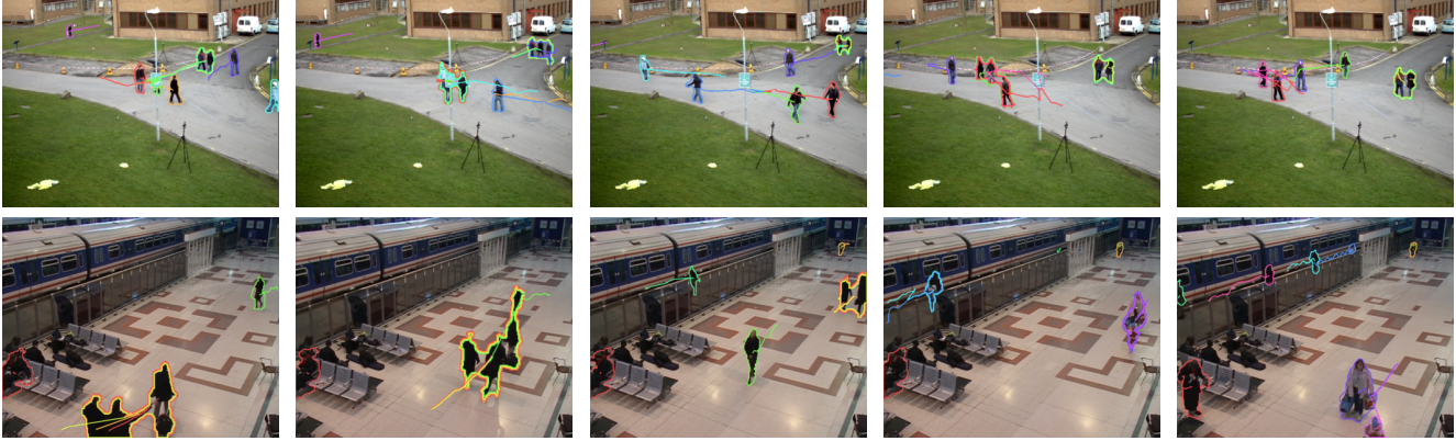
Figure 4. Tracking results for PETS'09 S2-L1 (first row) and PETS'06 S1-T1-C (second row). Identities are color-coded so this image is best viewed in color. Objects in a group are identified by nested outlines with their respective colors. Trails show the short-term trajectory of each object. Note that sudden changes in position are not tracking errors, but due to merged objects sharing the same position when in a group. Even though most tracks go through complicated interactions, reasoning about the formation of groups allows the tracker to recover their identities.
