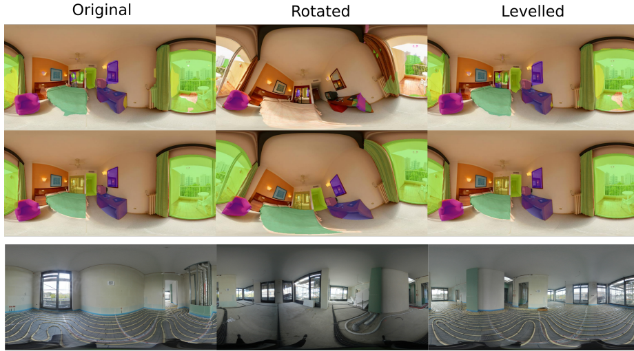
Fig. 8. Top row: Qualitative results for the downstream task of semantic segmentation (sec. 3.4). Middle row: Ground truth. The model performs well on the original images (left), but significantly worse on rotated images (center). Levelling with our method (right) recovers the performance. This highlights the importance of levelling for realistic downstream tasks. Bottom row: Example scenes from the construction dataset.
