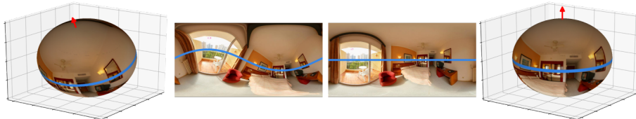
Fig. 1. Illustration of the problem of levelling spherical images. From left to right: a spherical image captured at a tilted angle relative to the sky (red arrow), with the horizon line shown in blue; its 2D representation (equirectangular image), with heavy distortions due to the rotation; the same image, undistorted by our system; the aligned spherical image in 3D.
